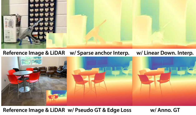
Figure 3. Effects on the synthetic data lidar simulation and real data pseudo GT generation with the edge-aware depth loss. The middle and right columns are the depth prediction results of our different models. The two rows highlight the significance of sparse anchor interpolation for lidar simulation and pseudo GT generation with edge-aware depth loss, respectively.
